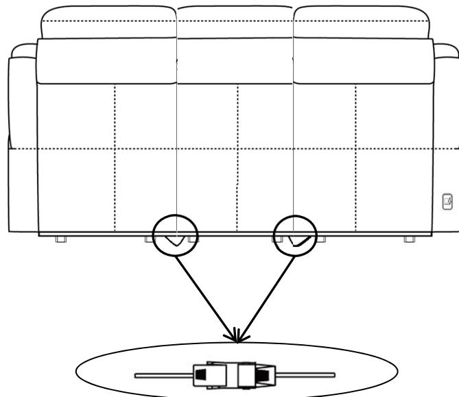
Step10: Plug power parts connection (refer to step 1) into socket at back panel of the left hand facing recliner, then Plug Recliner power cable into power source / wall.
